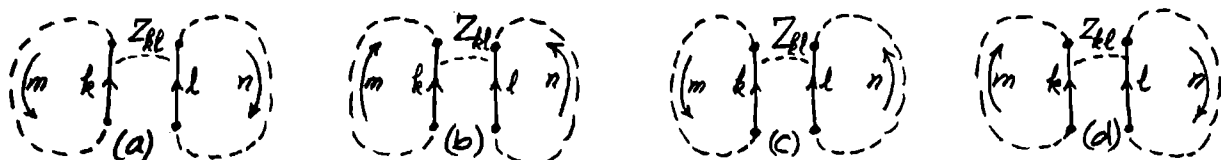
[k, m] Z_{kl} [l, n] = +Z_{kl} in (a) and (b). [k, m] Z_{kl} [l, n] = -Z_{kl} in (c) and (d).
