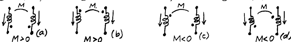
Fig. 2, exhibiting the rule of signs for mutual inductances.
